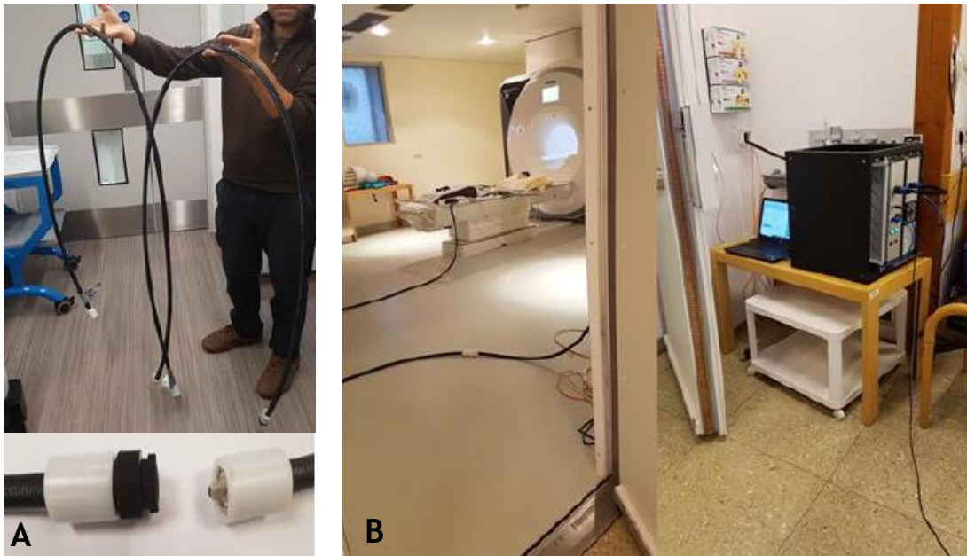
FIGURE 4. A) SECTIONS OF THE FLEXIBLE AXIS; B) PICTURE SHOWING HOW THE TRANSDUCER CONNECTS FROM INSIDE THE MRI TO THE MOTOR IN THE EQUIPMENT ROOM THROUGH THE FLEXIBLE AXIS.
