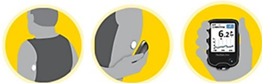
Figure 1: Apply sensor to arm, scan sensor with reader, reader displays current glucose level, glucose trend arrow and previous 8 hours of data.
